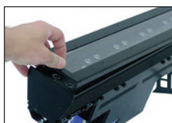
2.3 Insert the new VarioOptic. Apply the screws by hand.
