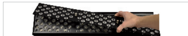
3.2 Carefully remove the optic modul and insert the new one and fix with screws.
